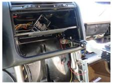
Reach in and remove the two upper screws of the heater core cover.
