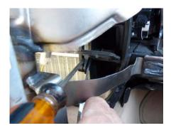
Unsnap both ends of the actuating arm (about 4" long, on the right side of the heater core) that operates the flap in front of the heater core. I used a screw driver to force the arm out of the two holes that the tabs go through.
