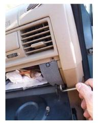
Remove 8 screws – two at the top inside the vents above the glove box, two just under the lip of the glove box door (covered by small covers – pry up with small screw driver), two above the hinge, and two underneath. The last two have larger washers, so keep separate.
