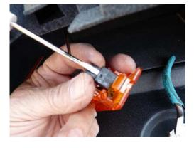
Remove the bolt (10mm socket needed) behind the light (if present.)
