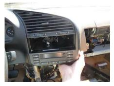
Three of them are almost impossible to reach, so here is how I did it. The top two are behind the heater/AC controller. Reach in behind and push it out. Press the release and unlatch the large blue connector. Pull straight out on the small black connector.
