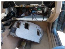
If the panel under the glove box hasn't been removed, remove it. You will need to unclip the light from the top side then pull it back through the hole.
