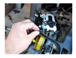
Lift (unsnap) the center shift console (with the "PRN321") and disconnect the Auto/Manual switch, then the small connector to the shift LEDs (Caution: the little circuilt board breaks off easy and the connector is hard to unplug.)
