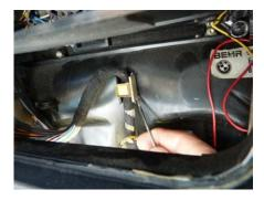
Pry the clip off the heater controller harness on the front of the heater core cover. I used a small screw driver on the side to release the two sharp teeth that grip the cover.
