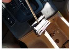
Remove the screw beneath the hazard switch. Leave the boot around emergency brake handle but unclip it from console. Pull the rear portion of the center console back to remove. Snake the emergency brake boot through the hole and remove the console. In the front half of the console, remove two screws at the top front of the console (they are vertical, below the Heater/AC controller.
