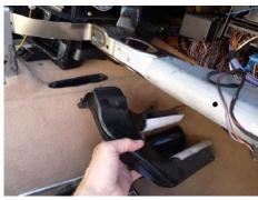
Reach in behind the heater housing and find the knob of the cabin air filter cover – it is barely visible. Turn it counter-clock-wise about 90 degrees and remove the cover. It may not unlatch or come out easily, be careful not to pull too hard as it will break the latch (ask me how I know, though it seems to still work properly.)
