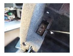
Unclip the flashlight holder with a small screw driver on both sides.
