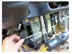
To remove the shaft that holds the flaps, pry the left side of the heater core housing to the left enough for the shaft bearing to come out of the housing. Pull the shaft away from the core and slide it to the left, taking the left flap and the shaft out, but leaving the right flap in place.
