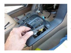
Reach under the black center of the console and pop up the switch groups. Grip the body of the connector and wiggle to unplug switches,
