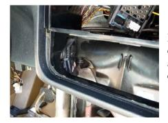
It is very difficult to work the cover out from under the dash. I found a molded cable bracket not being used, and in the way. I cut it off with a large pair of wire cutters.
