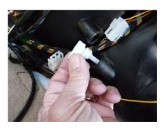
Remove the temperature sensors from the heater box – grip the edges of the connectors and unlatch the connectors from the two sensors.
