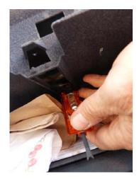
Remove the light inside glove box – pry behind the lens at the rear of the glove box to pop it downward. It and the built-in switch will fall downwards. Carefully unplug the
