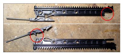
**4b)** Then inspect lifting gate arms for cracks. See image below (arms removed for clarity).
