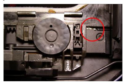
New cable trolleys come with matching toothed racks. They are sync'ed with trolley gear (see step10[e] below) and may be installed together. Once installed, re-install motor, ceiling liner (see step 10[e] below), and test.
