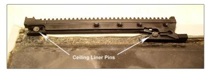
With sunroof mechanism in full open position, test liner for freedom of movement BEFORE attaching toothed racks. Liner has flexible edges which can be shaped to conform with curvature of frame. Don't be alarmed if liner doesn't always catch the slide rail slot when closing by hand. The sunroof's trim panel (#3, diagram 1) pinches the liner between it and the slide rail, holding the liner down as it moves.
