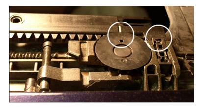
Once installed, detach rain gutter from lift gates by pressing outward on metal arms and pull rain gutter forward, clear of roof. Install ceiling liner between rain gutter and cable trolley, then slide liner forward to engage racks. Re-attach rain gutter and test liner movement.
