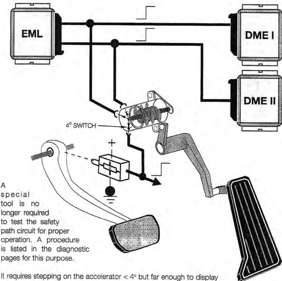
A special tool is no longer required to test the safety path circuit for proper operation. A procedure is listed in the diagnostic pages for this purpose.
