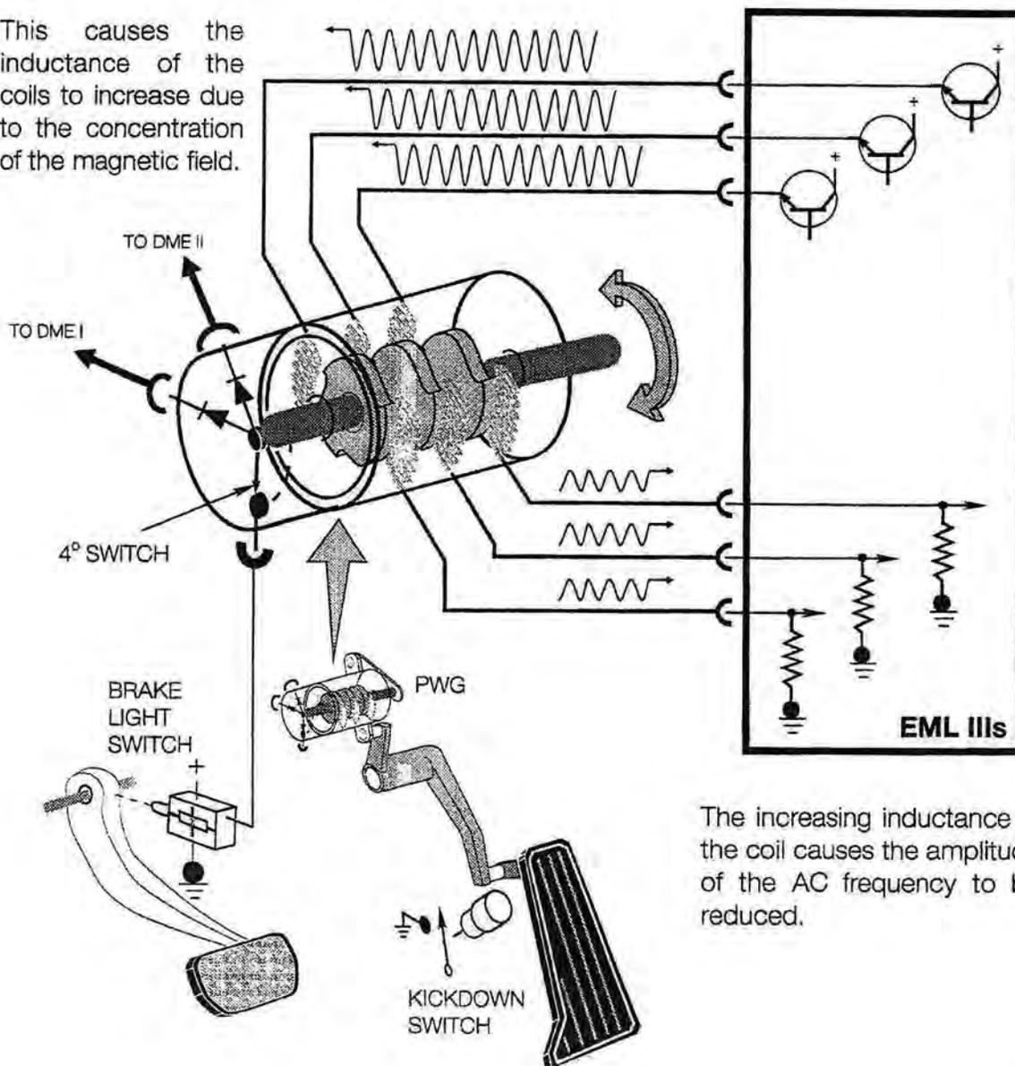
The increasing inductance in the coil causes the amplitude of the AC frequency to be reduced.
