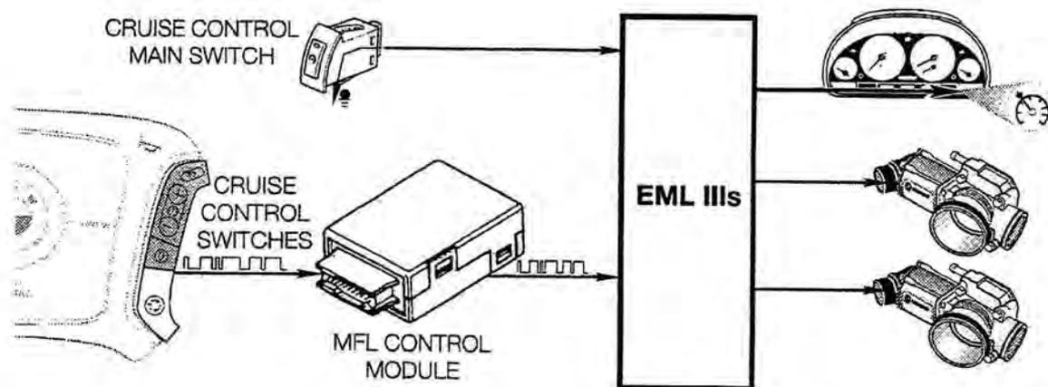
The EML controls the cruise control indicator lamp in the instrument cluster. When the main switch is pressed, the indicator lamp is illuminated.
