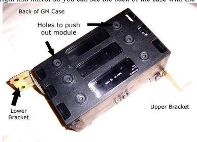
Slide the new module back in and replace all the connectors.
