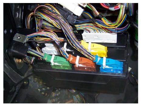
You see a white plastic vertical thing on the back of the blue connector. This is a "lever" that will move to the right. You see a little ridged tab looking thing just to the right of the white lever. Ok. get a little screwdriver and a bigger screwdriver. Take the little screwdriver and push down on the ribbed thingy a little, keep pushing a little, then take the bigger screwdriver and place it on the left side of the white thing and push to the right. The
