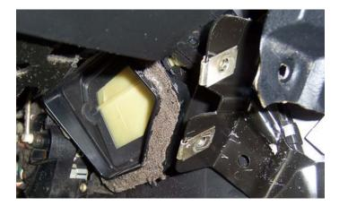
This picture shows the right bracket that holds the Knee-support. To remove that hidden upper bolt the bracket gets bent a little, but you can bend it back easily.
