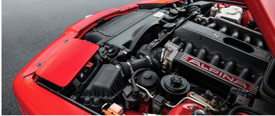
though-flow optimised, powder-coated intake system and a stainless steel exhaust system with stainless steel exhaust manifolds and metal catalysators, the 2-valve engine attains optimum thermodynamic efficiency. With these technical refinements, the twelve-cylinder
