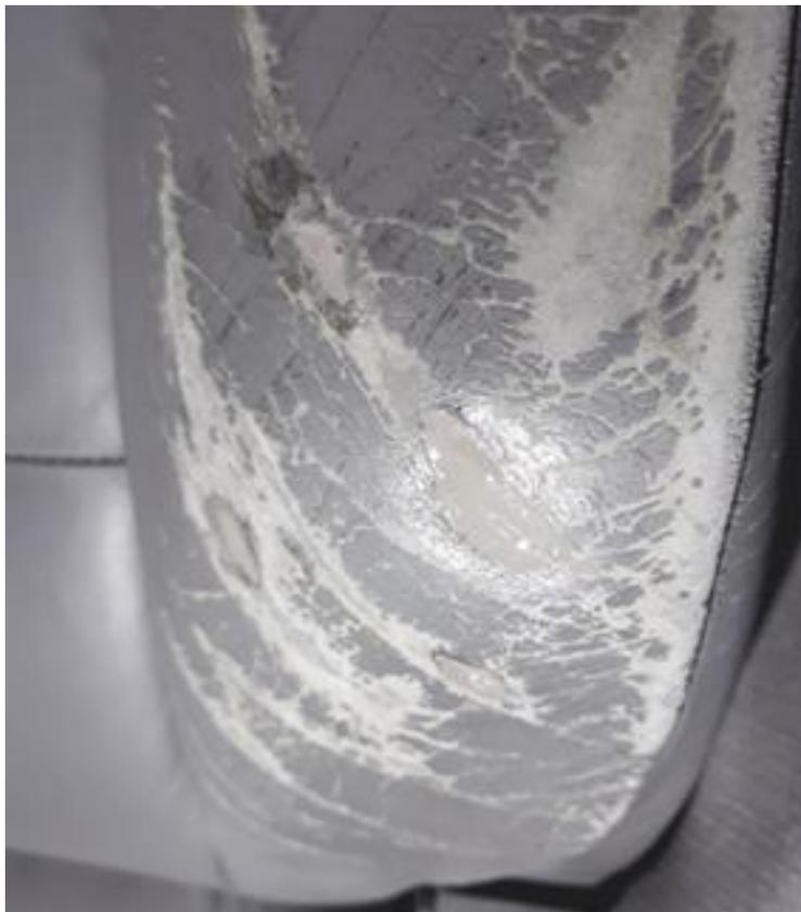
the Leatherique Crack Filler, the Colourlock Fluid Leather can be ordered in the matching color, sets up fairly quickly, and is not water soluble. It does settle and sink requiring multiple applications to build up to surface level. I then spread Fluid Leather over the entire worn areas using a thin putty knife followed by smoothing the surface with the GLD pen. It's filled with some type of solvent in a container similar to a large felt pen with a wide flat tip.
